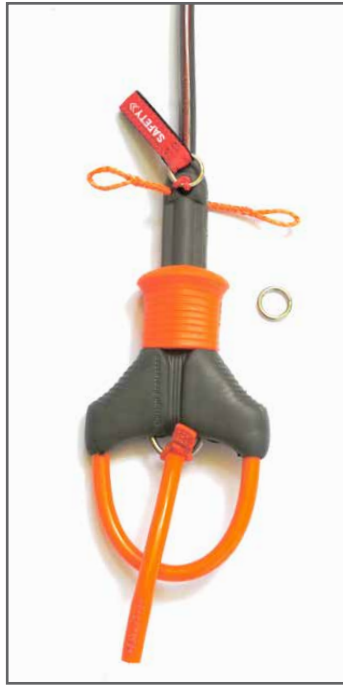
2. Feed the suicide connector through the hole in the buffer.
